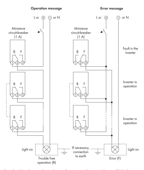
Figure 5: Wiring diagram with several inverters for connection of operation indicator and fault indicator (example)
