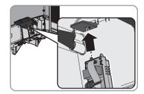
4. Lead the ribbon cable upwards behind the display.
