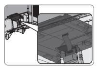
Fasten the multi-function relay using the washer and the cheese-head screw (torque 1.5 Nm). For this purpose, use an Allen key (AF 3).
