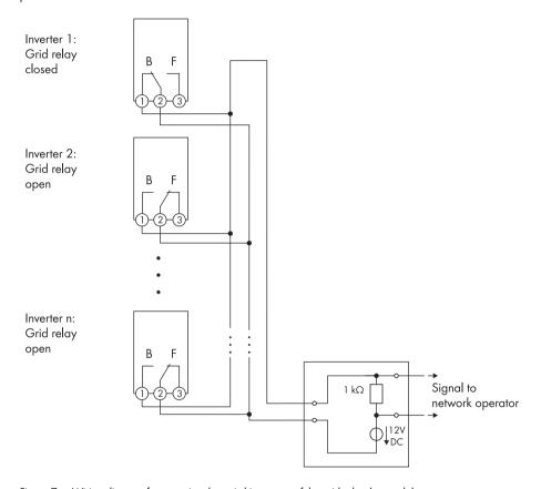
Figure 7: Wiring diagram for reporting the switching status of the grid relay (example)
