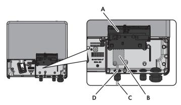
Figure 4: Installation area and cable route in the Sunny Boy/Windy Boy with the lower enclosure lid open and the display flipped up
