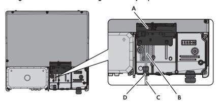
Figure 3: Installation area and cable route in the Sunny Tripower with the lower enclosure lid open and the display flipped up
