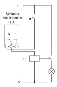
Figure 6: Wiring diagram for connection to control a load or for the power-dependent charging of the batteries
