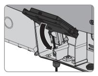
7. Fasten the screw of the display hand-tight.
