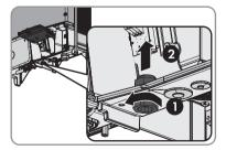
Insert the cable gland from the outside into the enclosure opening and tighten it from the inside using the counter nut.
